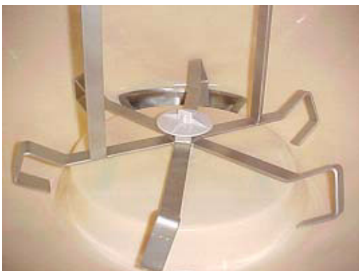
Figure 6. Agitator with Ice Slide Installed
