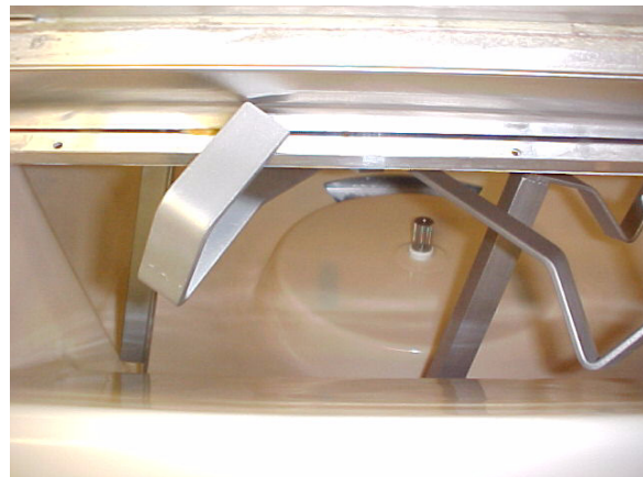
Figure 3. Hook Agitator to Front Lip of Adapter
