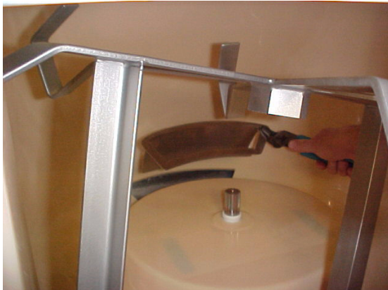
Figure 4. Position Ice Slide Inside Hopper
