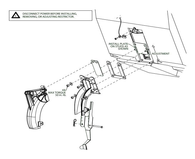
Figure 1. Gate Restrictor Plate
