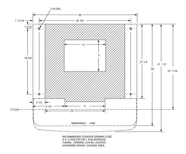
Figure 2. IDC 2XX Mounting Template
