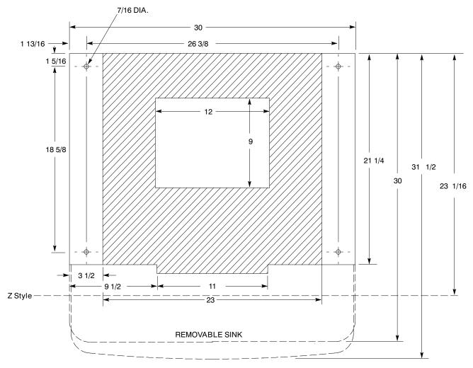
RECOMMENDED COUNTER OPENING SIZE 9 X 12 FOR UTILITIES AND BEVERAGE TUBING. OPENING CAN BE LOCATED ANYWHERE WITHIN SHADED AREA.
