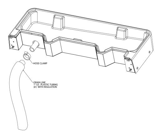
Figure 7. Drip Tray Drain Assembly
