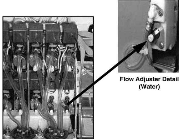
**Figure 3. Valve with Flow Adjusters**
