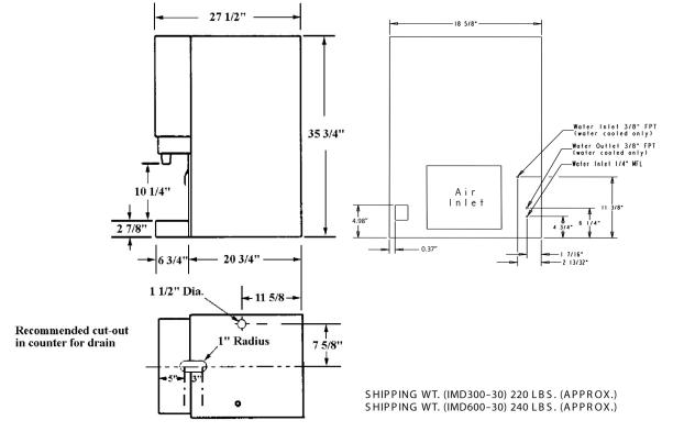
Figure 2. Dimension Drawings (30 lbs.) IMD 300-30 and IMD 600-30
