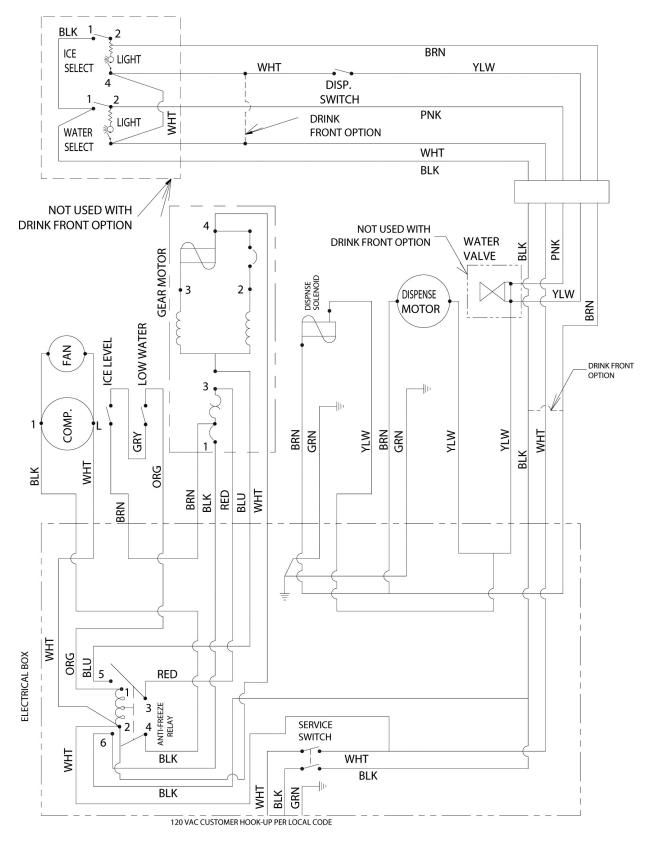
Figure 16. . Schematic IMD 300-15
