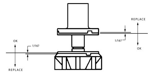
Figure 5. Upper Bearing and Auger Assembly
