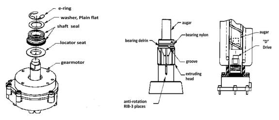
Figure 7. IMD 300 Shaft Seal
