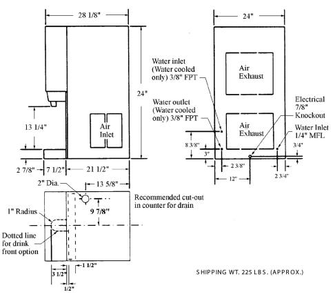
Figure 3. Dimension Drawings (90 lbs.) IMD 600-90
