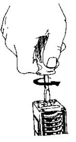
Figure 6. Adjustment Screw
