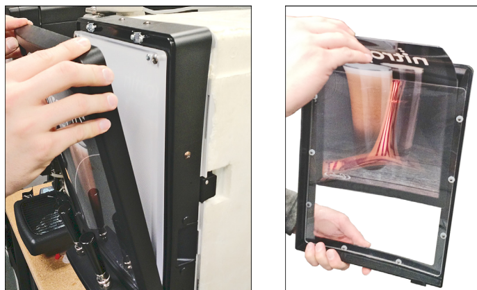
Figure 2-1 - Front LED-Backed Merchandiser Removal
