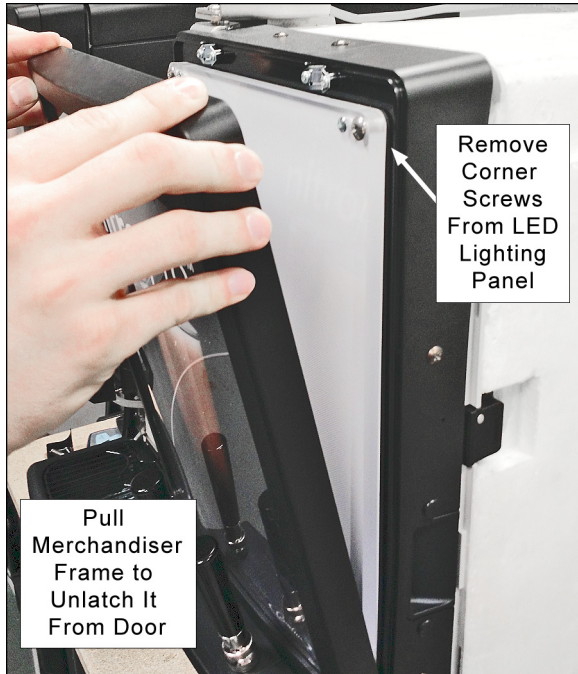
Figure 6-10 - Merchandiser LED Backlight Removal
