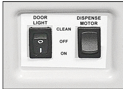
Figure 3-17 - Front Door Switches
