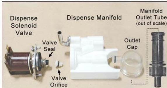
Figure 6-6 - Dispense Manifold Assembly
