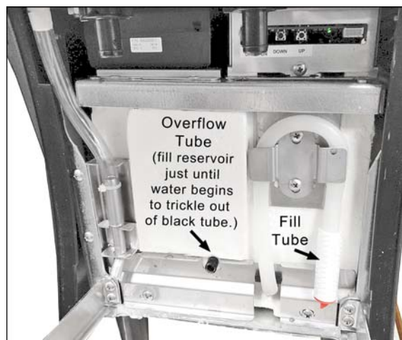
Figure 4-2 - Ice Bank Fill & Overflow Tubes
