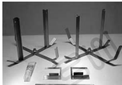
Figure 21. For 22" and 44" wide units special agitators are used in place of the diverter.
