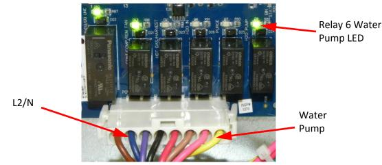
When verifying voltage out of Board, check at the Blue and Yellow wires.
