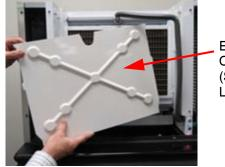
Evaporator Cover (Slide up and Lift Off)
