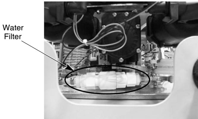
**Figure 40. Water Filter Location**
