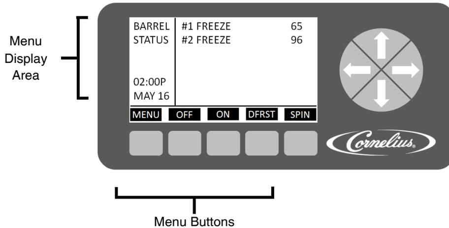
**Figure 11. Control System Display**
