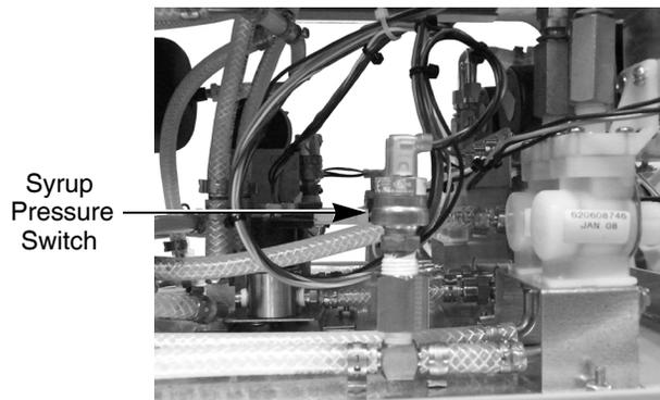
**Figure 53. View of Syrup Pressure Switch and Valve**
