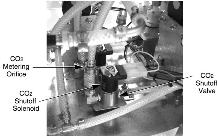
Figure 47. Side View of CO<sub>2</sub> Shutoff Solenoid (2 Barrel Unit)
