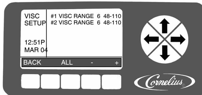
**Figure 22. Viscosity Setup Screen**
