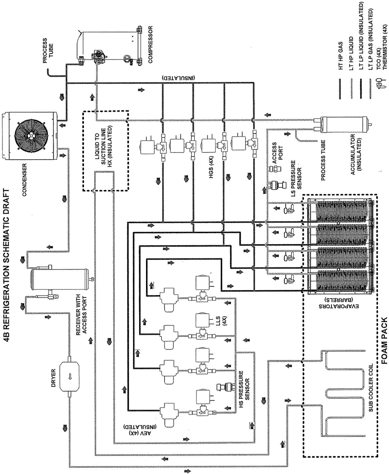
Figure 3. Viper System 4-Barrel Refrigeration Schematic
