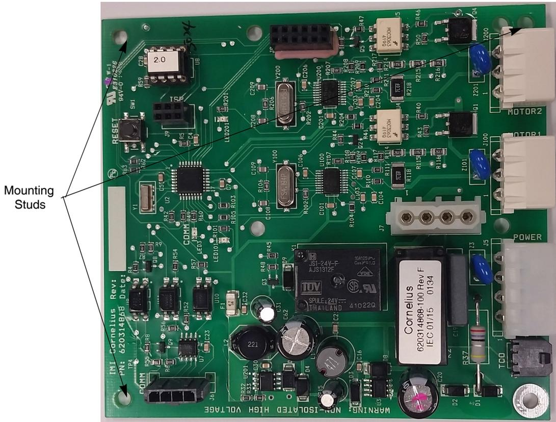
Figure 57. View of Motor Board in E-Box
