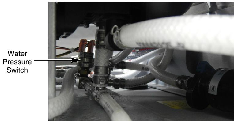
Figure 54. View of Water Pressure Switch
