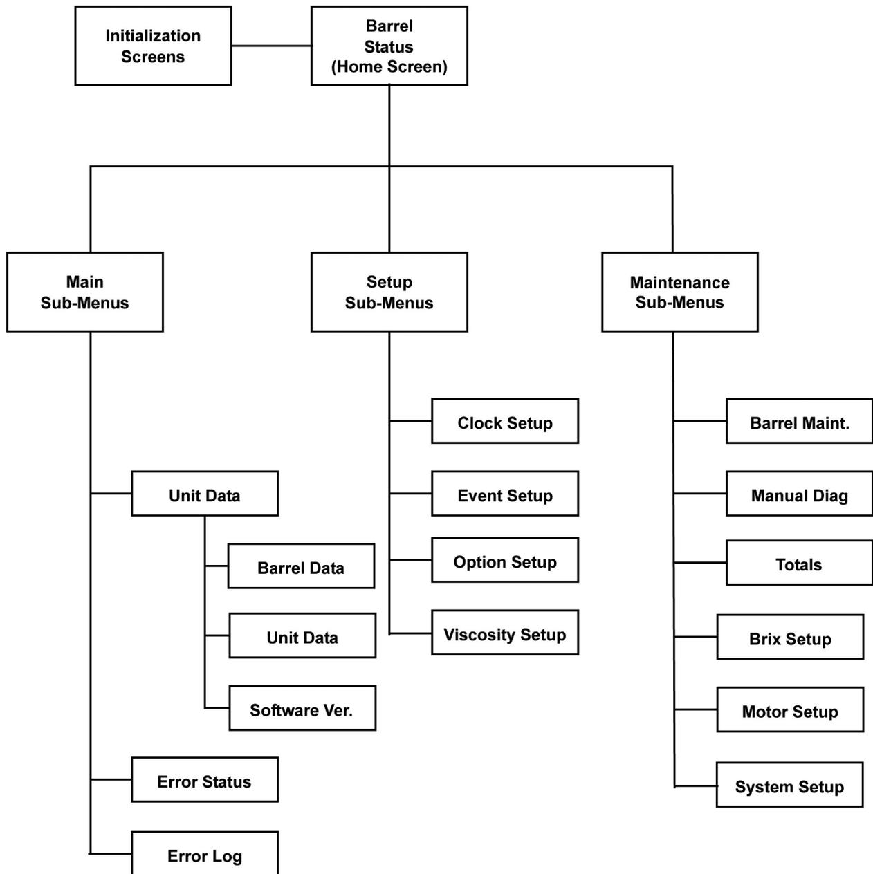
Figure 12. Software Structure
