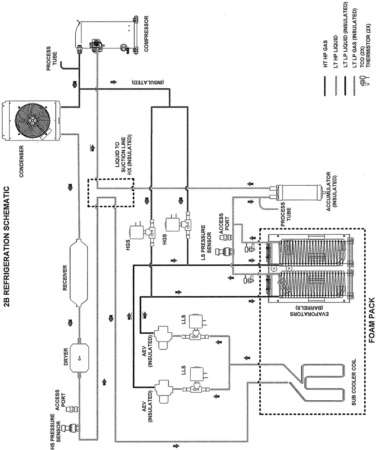
Figure 1. Viper System 2-Barrel Refrigeration Schematic
