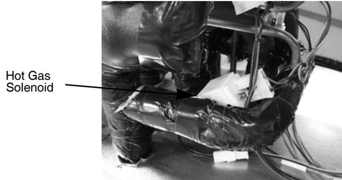
Figure 51. Hot Gas Solenoid (1 per barrel)
