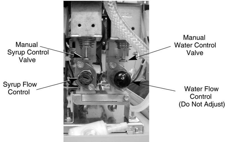
Figure 32. Flow Controls
