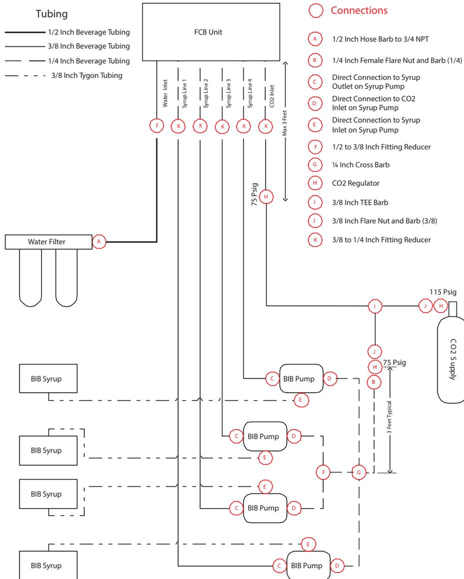
Figure 7. Cylinder CO<sub>2</sub> Connection
