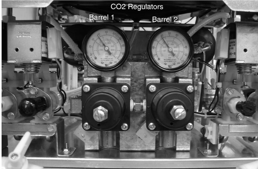
Figure 49. Front view of CO2 Regulators w/ Access Panel Removed (2 Barrel Unit)
