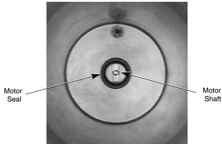
Figure 41. Front View Inside of Barrel w/ Faceplate off
