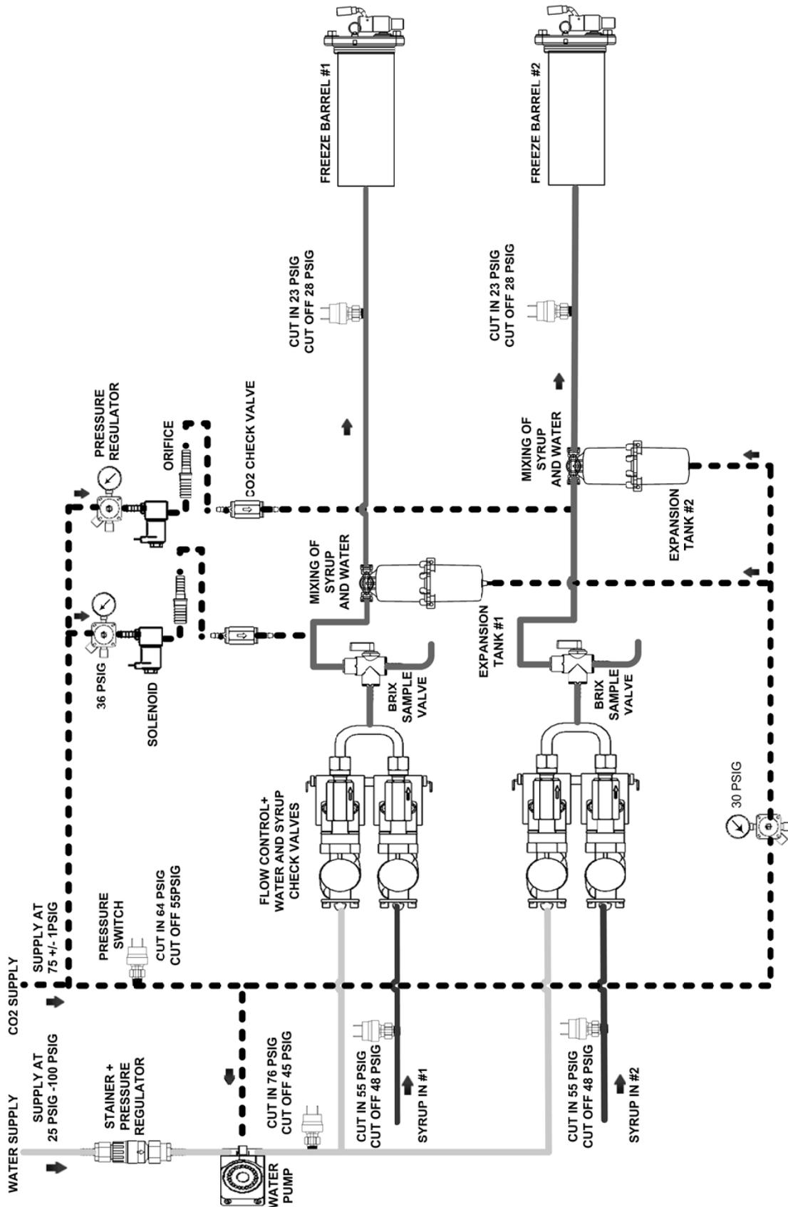
Figure 8. 2-Barrel System Schematic
