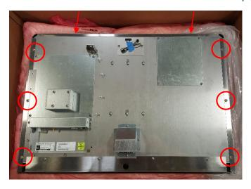
Step 2: Remove the four screws for the touch controller cover, remove cover, and set aside.
