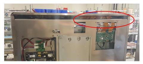
Step 5: Slide the new glass wrapper assembly onto the door chassis, taking special care to slip the touch sensor ribbons through the same gap as the original ribbons. CAREFULLY insert the touch sensor ribbons on the touch controller and lock in place. Complete the previous steps in reverse order to finalize reassembly.
