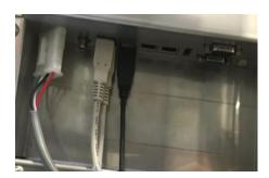
First, open the unit's door. On the back of the display, unplug the black USB connection and plug in your USB flash drive.
