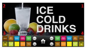
Tap each corner of the video screen starting in the upper right corner. Continue to each corner in a counterclockwise direction, in the form of a "C". The screen will flash white when you touch corners.
