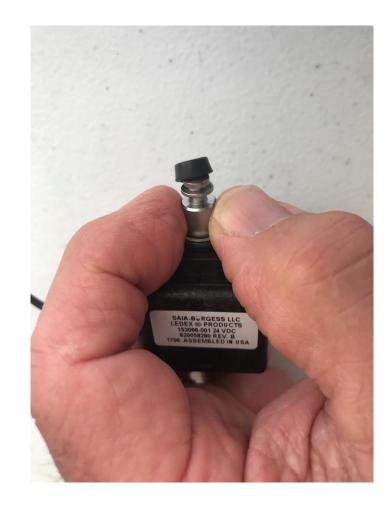
Insert the solenoid back into the valve and rotate ¼ turn clockwise to lock it in. Also, ensure that the coils and wires are in their original orientation.
