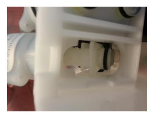
Start the solenoid at a 45 degree angle and ensure that the rear flange of the valve fits behind the wall of the valve bank. The valve should slide easily into place, do not force it.
