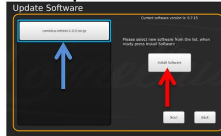
The IDC Pro will recognize the software file from your inserted USB flash drive. Ensure the software file on the left of the screen is selected and highlighted in blue.
