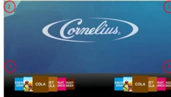
Tap each corner of the merchandiser screen in a counterclockwise direction, starting in the upper right corner to form a "C."
