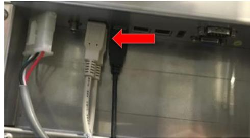
On the back of the digital merchandiser, unplug the black USB connection and plug in your USB flash drive containing the software update file.
