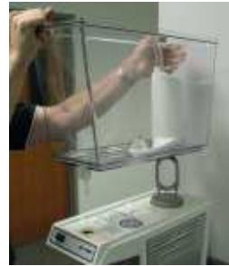
Remove the concentrate drain by squeezing both sides and pulling straight down. Remove the pump housing by squeezing the sides and lifting it off, then remove the impeller and pin by pulling them out of the housing. Lift the bowl gasket off of the bottom of the bowl.
