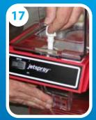
When properly seated, the bowl will lie flat on the base. Push the handle back and insert the pinch tube.
