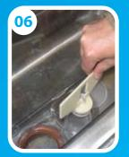
Remove the impeller by pulling straight up.
