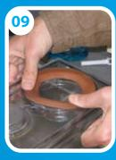
Insert the gasket into the bowl base and smooth with thumbs until the gasket is flat in bowl groove.
