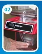
Push back on the handle to release the pinch tube and bowl from the base.
