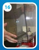
To re-mount the bowl assembly, place the bowl over the evaporator and lower. Be sure that the push handle is pulled forward.
