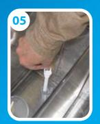
Remove the pinch tube by pulling straight up.
