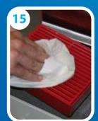
Wipe down the drip tray with a clean damp cloth. Repeat steps 8 through 15 with an appropriate sanitizer solution.
