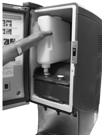
**Figure 5. Loading a Concentrate Container**
