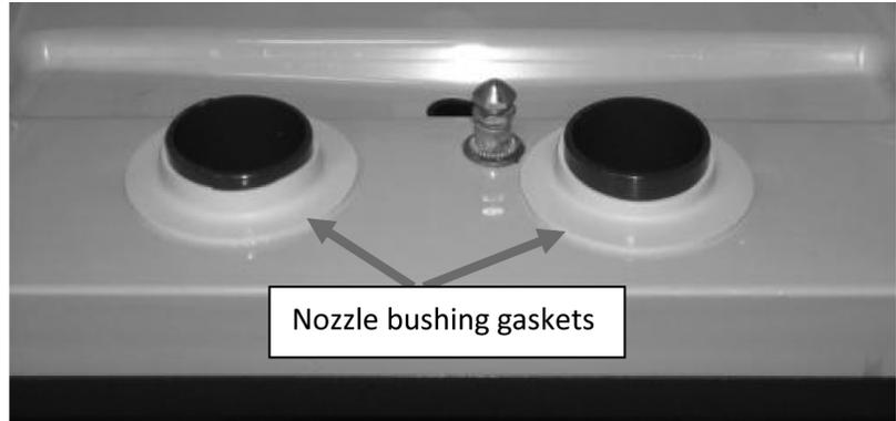
**Figure 17. Nozzle bushing gaskets - proper installation**
