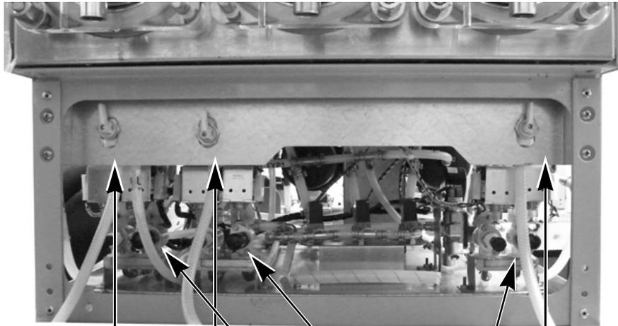
Product Supply Valve Barillet 1      Product Supply Valve Barillet 2      Flow Controls Barillet 1      Flow Controls Barillet 2      Flow Controls Barillet 3      Product Supply Valve Barillet 3
