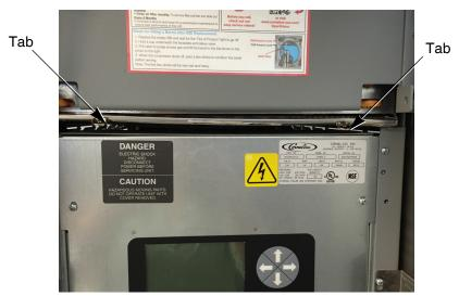
Figure 37. Air Filter Location
