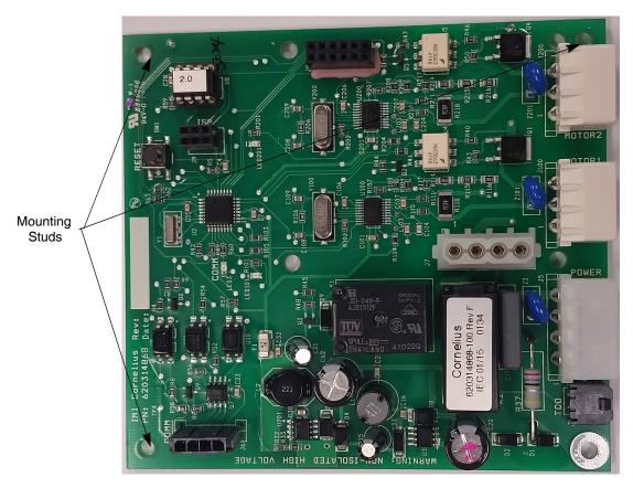
Figure 57. View of Motor Board in E-Box
