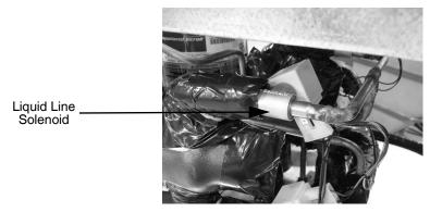
Figure 52. Liquid Line Solenoid (1 per barrel)
