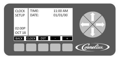
Figure 19. Clock Setup Screen
