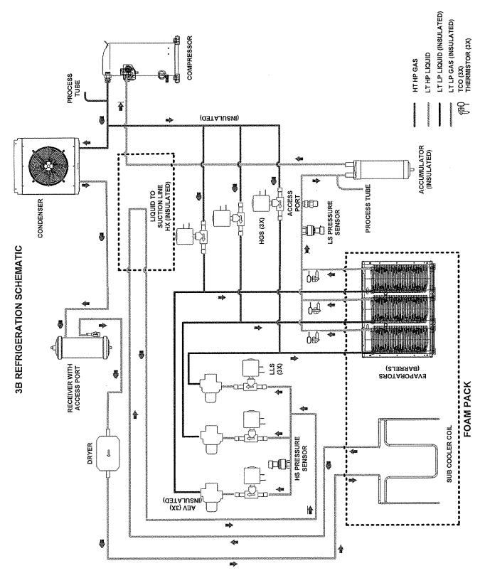
Figure 2. Viper System 3-Barrel Refrigeration Schematic
