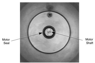
Figure 41. Front View Inside of Barrel w/ Faceplate off
