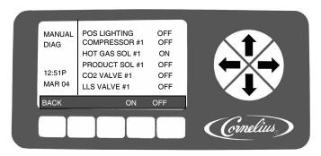
Figure 26. Manual Diagnostic Screen
