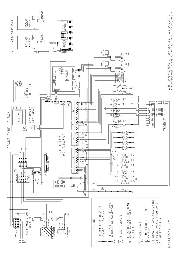
Figure 4. Viper 2-Barrel Wiring Diagram (W/Transducer)
