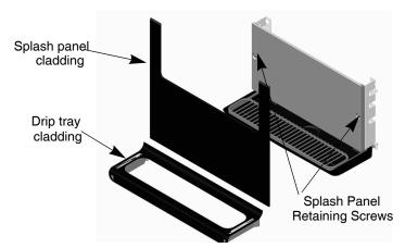
Figure 30. For Carbon Splash Panel Mounting Screws
