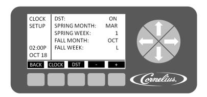
Figure 20. Daylight Savings Setup Screen
