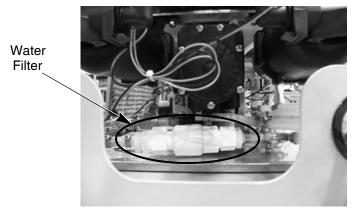
Figure 40. Water Filter Location
