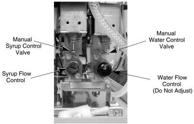
Figure 32. Flow Controls
