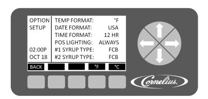
Figure 23. Option Setup Screen
