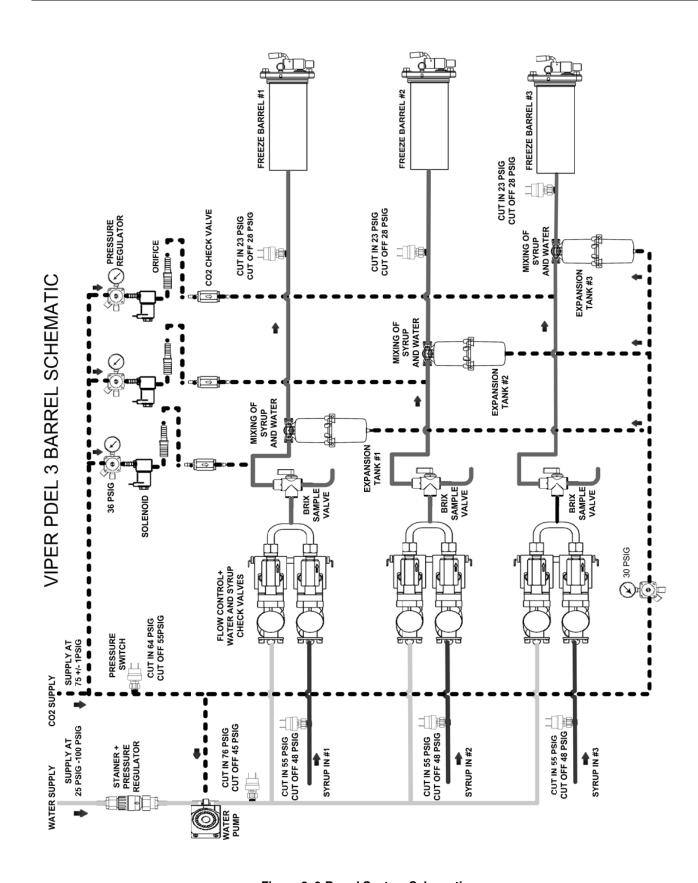
Figure 9. 3-Barrel System Schematic
