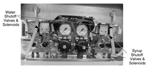
Figure 48. View of Shutoff Solenoids w/ Access Panel Removed (2 Barrel Unit)
