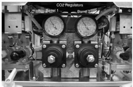
Figure 49. Front view of CO<sub>2</sub> Regulators w/ Access Panel Removed (2 Barrel Unit)
