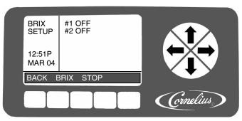
Figure 28. BRIX Setup Screen
