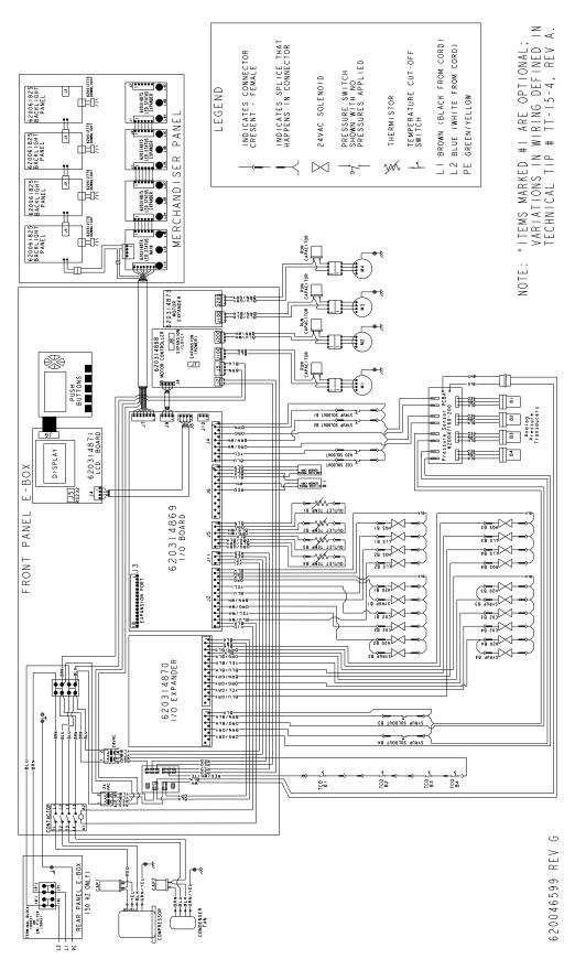
Figure 6. Viper 4-Barrel Wiring Diagram
