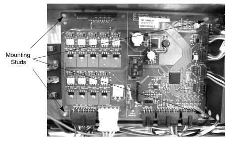
Figure 56. View of Control Board in E-Box
