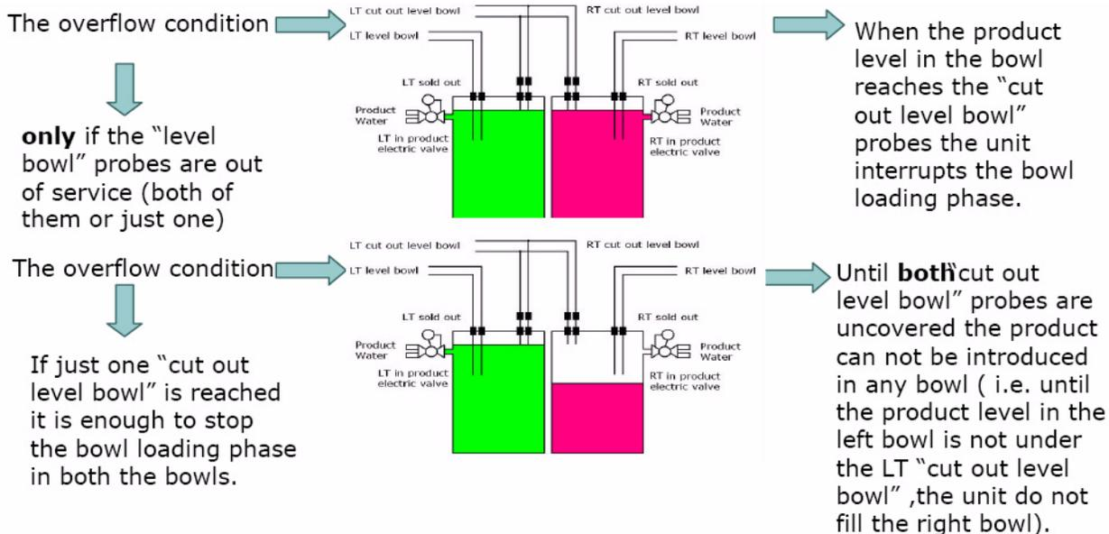
The "pressure and level control board" INDIRECTLY detects the lack of product because when the "sold out" pressure switch, set on the electro-valve, has detected the product missing, it stops the mix dispensing. In this situation the "level bowl" probes will never be covered, so after 1 minute (set time) the "pressure and level control board" detects the lack of product and the led (out of product) on the front panel is lit.
