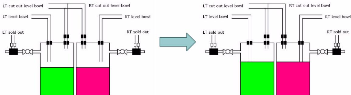
The "sold out" probes detect the product presence (or not) in the external tanks with a hysteresis of 3 seconds. 3 seconds software hysteresis are introduced to prevent the probes recognize the tank bowl conduit as empty when there is residual gas in it.
