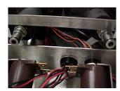
11. Reconnect all solenoid wires. Connect wires that used to be connected to the push button switches to the microswitches on the valve assemblies. The wires for the solenoinds and switches are numbered. Valve 1 is on the far left-hand side.
