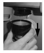
Replace with the Splitter Nozzle by pushing up and rotating right. 2.
