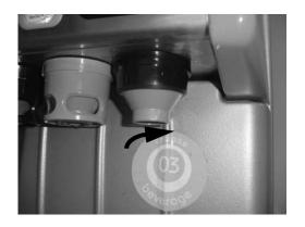
Insert the S tube into the Splitter Nozzle on the syrup tube you want to ratio.
