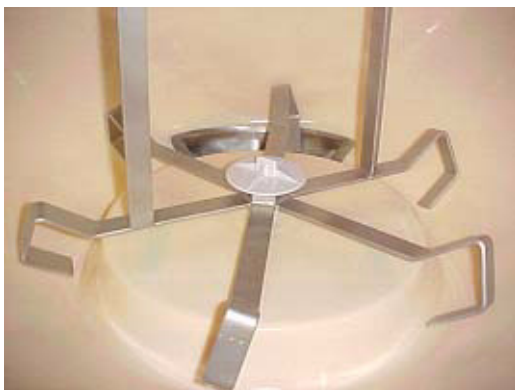
Figure 6. Agitator with Ice Slide Installed
