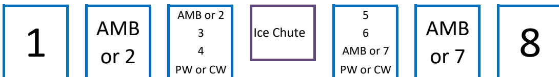
Enduro 150 Eight Line Coldplate with Two Prism Valves (10 Brands - 8 Chilled & 2 Ambient)
