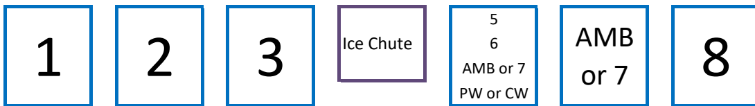
Enduro 150 Eight Line Coldplate with One Prism Valve (8 Brands - 7 Chilled & 1 Ambient)
