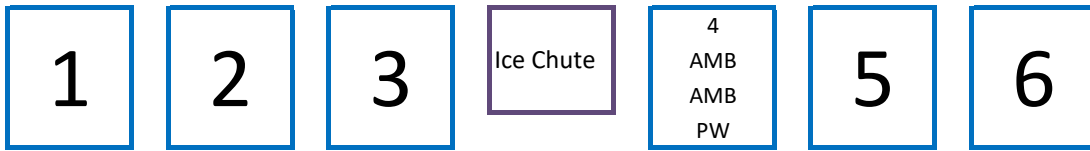
Enduro 150 Six Line Coldplate with One Prism Valve (8 Brands - 6 Chilled & 2 Ambient)
