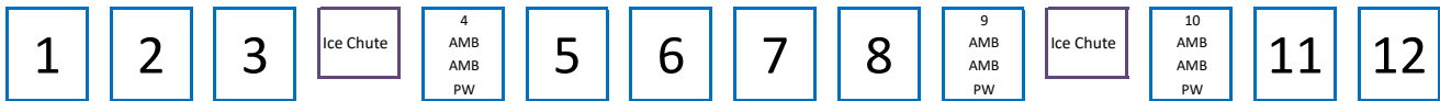
Enduro 300 Dual Six Line Coldplates with Three Prism Valves (18 Brands - 12 Chilled & 6 Ambient)
