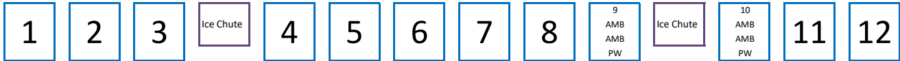
Enduro 300 Dual Six Line Coldplates with Two Prism Valves (16 Brands - 12 Chilled & 4 Ambient)
