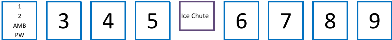
IDC 255 ProGate Ten Line Coldplate with One Prism Valve (10 Brands - 8 Chilled & 2 Ambient)
