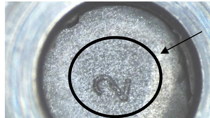
New Tip-P/N 620070041: Circle around the cavity number
