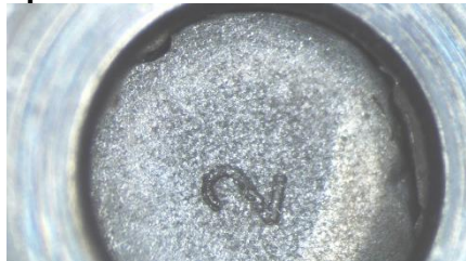
Current Tip-P/N 620711131: No Circle around the cavity number
