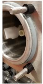
NOTE: Install Faceplate Spacers to prevent potential barrel damage and align the Faceplate evenly on the barrel's 4 threaded rods. The Faceplate Spacers are part of a kit or can be acquired individually; see below for all available configurations.
