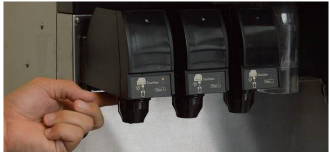
Finger shown to block sensor window and go into cleaning mode.
