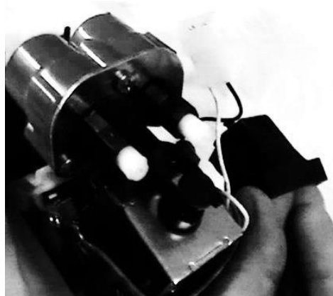
Step 2: Slide cover forward to remove.
