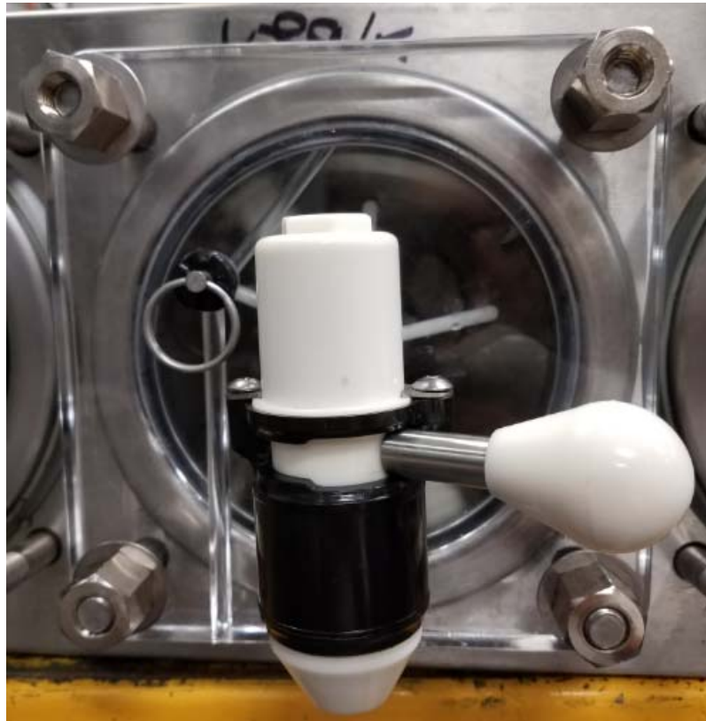
Figure 1 – Misaligned Faceplate (Bottom Nuts Overtightened). Motorman Valve Shown, but Applicable to all Valve Variations.
