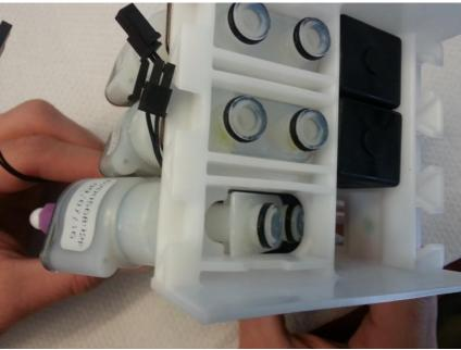
Ensure that the bottom red o-rings seat and are not pinched in the outlet barbs.
