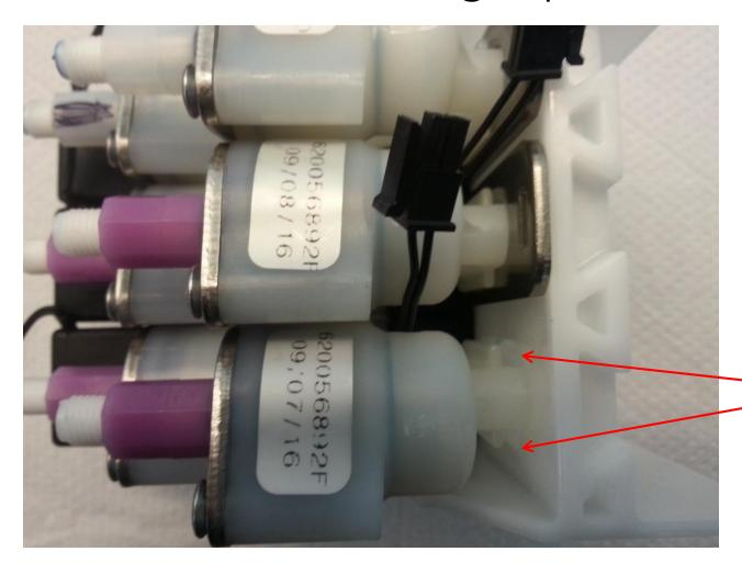
Insert locking clip into the gap between the valve bank and valve. If it doesn't slide in easily, the valve may not be aligned.
