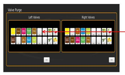
The valve layout on the screen is laid out the same orientation of the physical valves. If you were to take the valve purge screen and lay it over the valves it will show you what valve is what. EX: you are working on valve CW1; it is the 6<sup>th</sup> valve from the left on the top.
