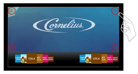
1. Display the keypad screen by tapping each corner of the video screen starting in the upper right corner and continuing to tap each corner in a counterclockwise direction, in the form of a "C".
