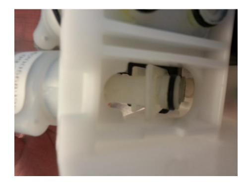
Start the solenoid at a 45 degree angle and ensure that the rear flange of the valve fits behind the wall of the valve bank. The valve should slide easily into place, do not force it.
