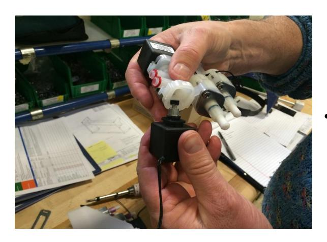
Use caution when removing and replacing spring so you won't lose or bend it Insert the solenoid back into the valve and rotate ¼ turn clockwise to lock it in. Also, ensure that the coils and wires are in their original orientation.
