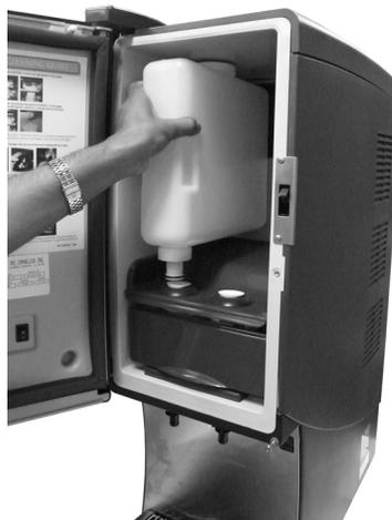
Figure 4. Loading a Concentrate Container
