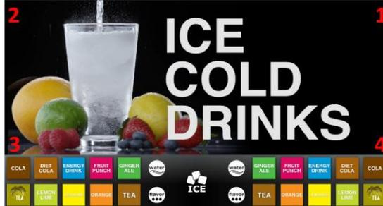
Tap each corner of the video screen starting in the upper right corner. Continue to each corner in a counterclockwise direction, in the form of a “C”. The screen will flash white when you touch corners. Wait for the video to reappear before proceeding to the next touch point.
