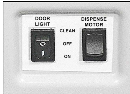
Figure 3-17 - Front Door Switches
