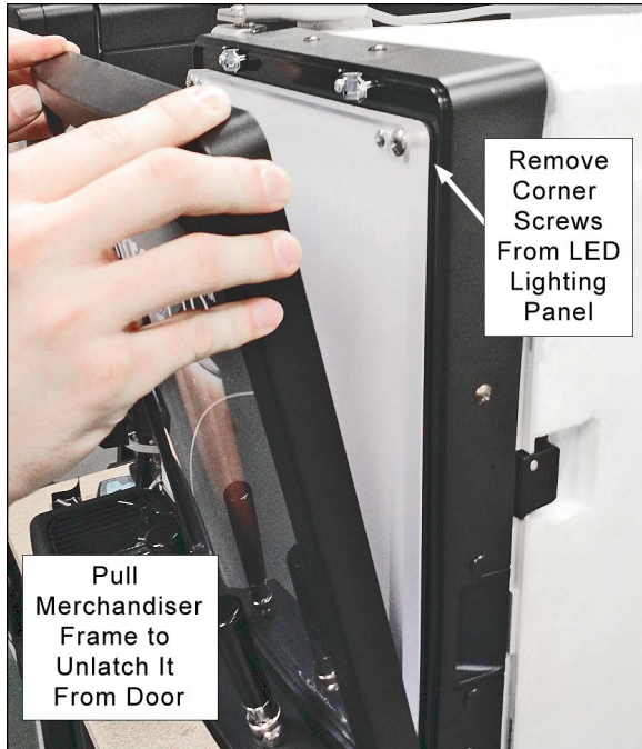
Figure 6-10 - Merchandiser LED Backlight Removal
