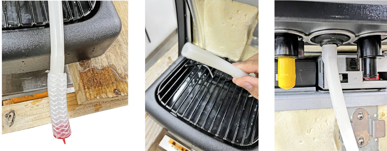
Figure 8. Bath Refill Tube Connection to Water Dispense Faucet
